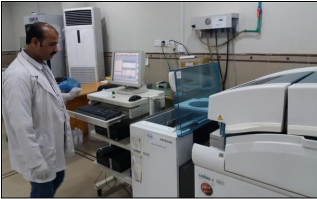
Fig 2: Showing the Hitachi Cobass 600 Fully Auto Analyzer (Used for LP and HDL, LDL, TG), Urea, Creatinine, HBA1C.
