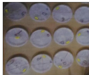
Fig 3: Filter paper contact test set up
