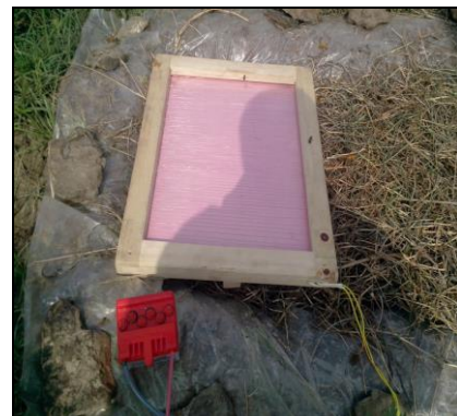
Fig 5: Venom collector device at field
